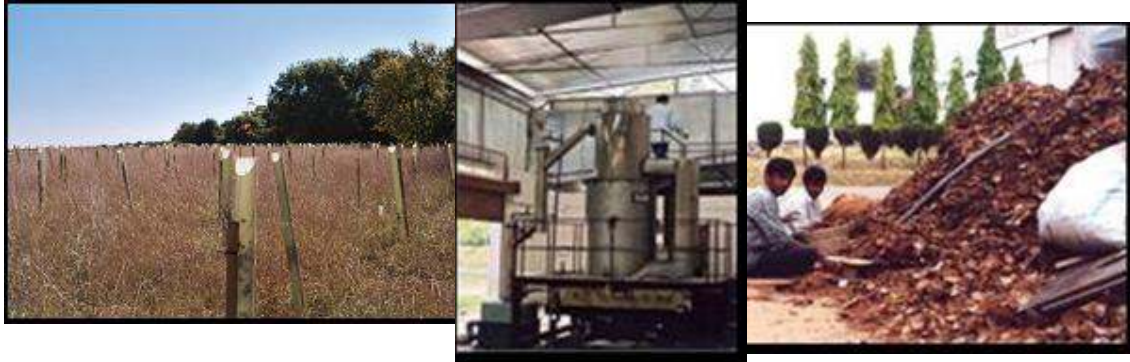
Figures 9 & 10. Coconut husks are used to power this Gasifier in India
